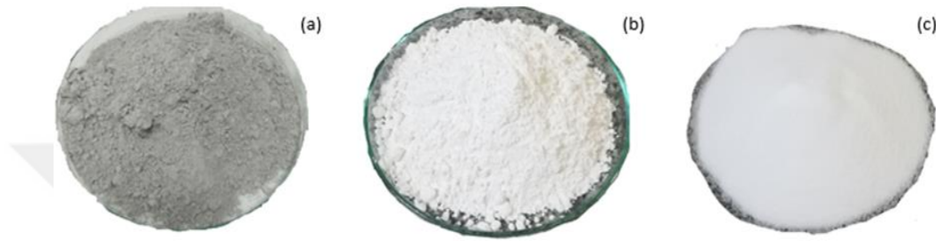
Figure 6.2 Pictures of (a) refractory powder (b) titania powder and (c) alumina powder (Personal archive, 2020)
