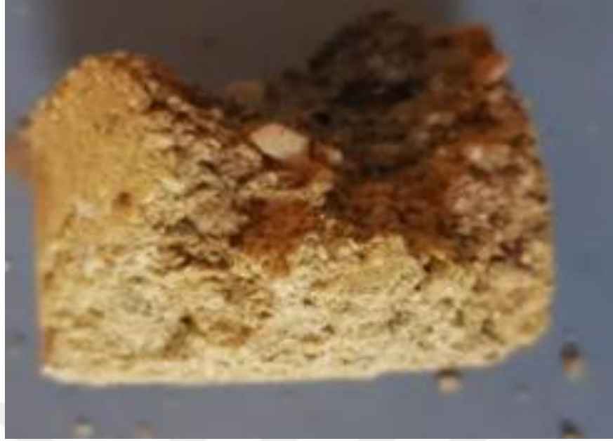
Figure 7.3 Disintegrated corrosion test sample sample with graphite (Personal archive, 2020)
