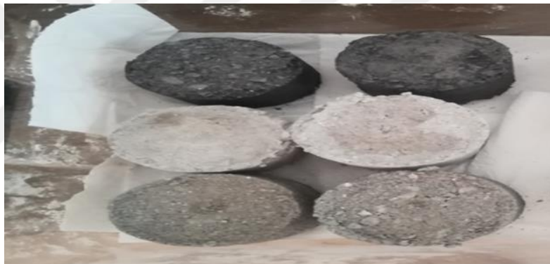
Figure 6.6 Pressed thermal shock test samples (Personal archive, 2020)
