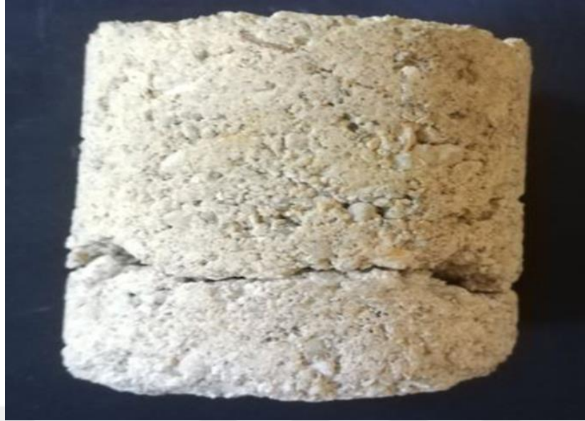
Figure 7.1 Cylindrical test piece after thermal shock testing (Personal archive, 2020)
