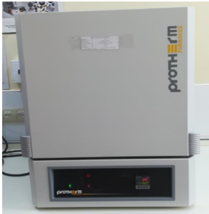
Figure 6. 3 Furnace using of sintering samples (Personal archive, 2020)
