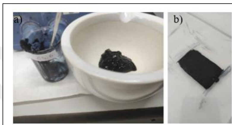
Figure 3.11 5% PEDOT: PSS/ 10% \text{Ag}_2\text{Se} solution and film (Personal archive, 2022)
